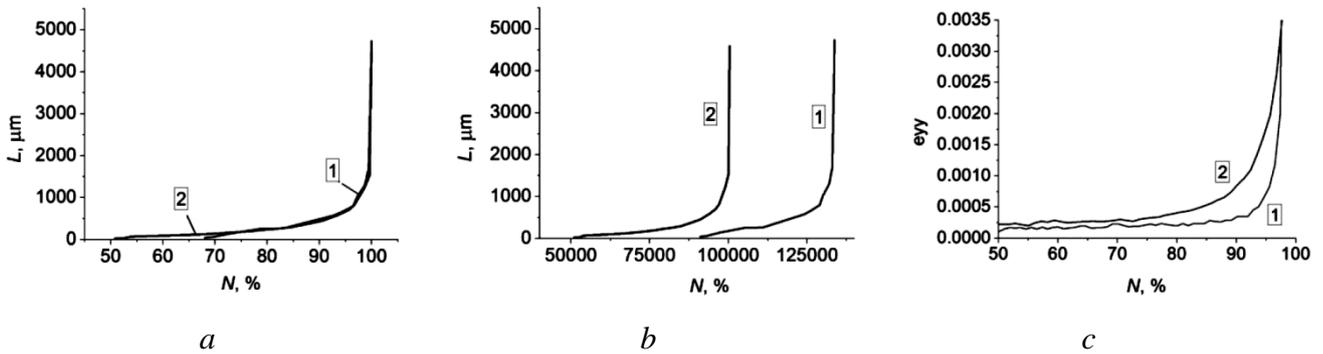
Fig. 2. Diagrams of fatigue crack growth versus *a*) the normalized number of cycles, *b*) the absolute number of cycles; *c*) dependences of longitudinal strain on cyclic loading (in percent prior to failure); 1 – emergency stock; 2 – after long-term use
